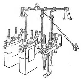
FIG. 112. A three-phase oil-break switch, with one oil cell removed.
